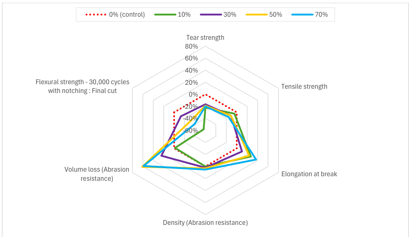
Figure 30 : Variations in the properties of the material samples incorporating different rates of SBS RRM compared to the properties of the control sample
